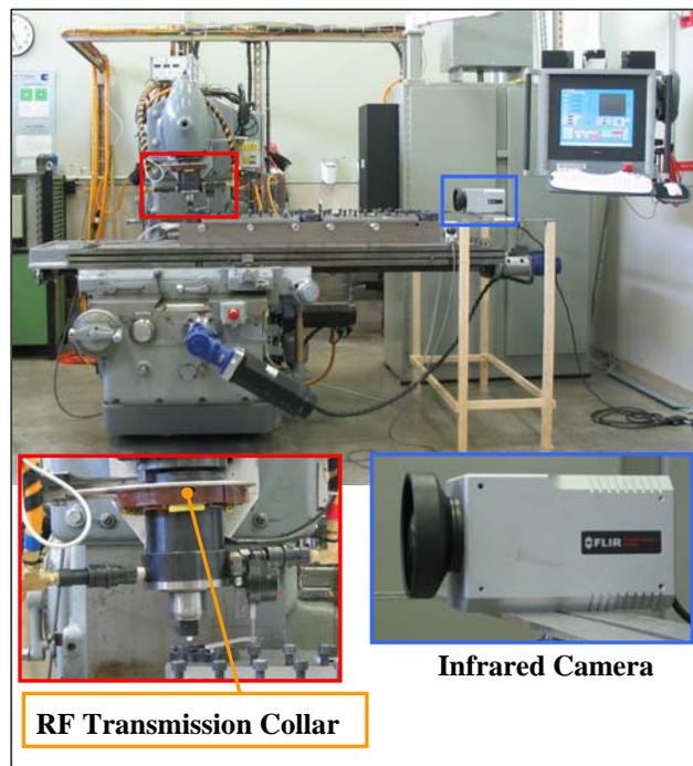
**Figure 1**—FSW facilities at BYU with temperature sensing equipment
