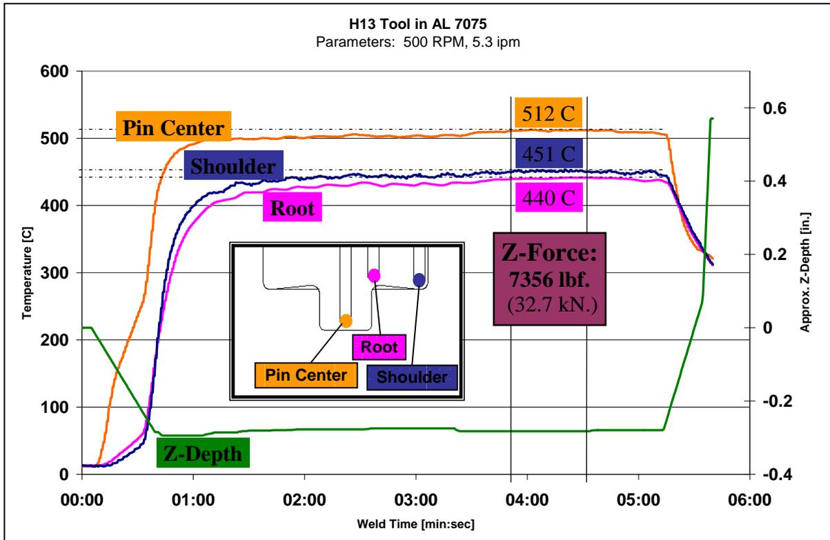
Figure 2—Plot of tool temperature and approximate tool depth versus time for a weld in 7075 Aluminum
