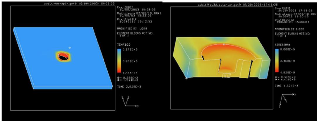
**Figure 1**—A two-dimensional slice, shown at the left, of the temperature distribution during the FSW process at  $t=3.535$  ms, modeled with a prescribed rotational boundary surface representing the tool. A cut away view, shown at the right, of the three-dimensional Von-Mises stress distribution of an Eulerian model, with a prescribed rotational condition on the surface representing the tool. Total time elapsed 1.37 ms.
