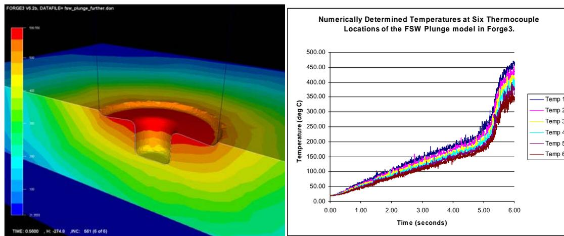
**Figure 2**—A cut plane view, left, of the Forge3 model of the temperature profiles at 6 seconds. The tool has been removed to allow the reader to view the shoulder
