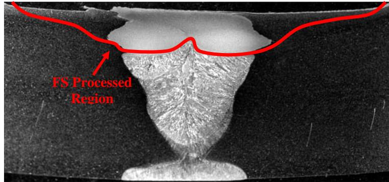
Figure 1 Macrograph of FS Processed Arc Weld
