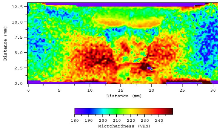
**Figure 3 Microhardness Map of FS Processed Arc Weld**
