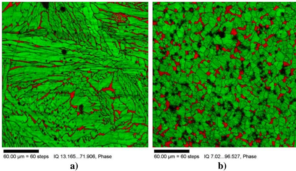
Figure 2 a) Continuous Ferrite Stringers in Arc Weld b) Refined Ferrite in FS Processed Region
