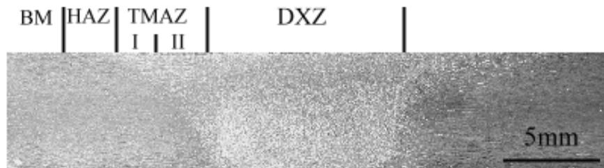
Figure 1. Cross section of the 7050 friction stir weld, showing the different region from base metal to DXZ.
